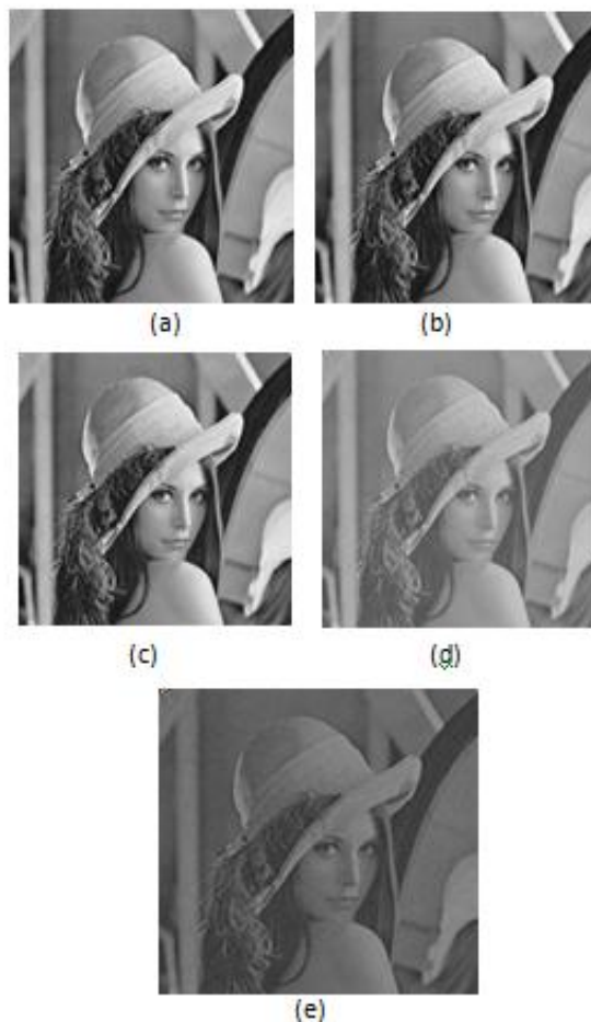
Fig. 4: Stego Images of DCT Steganography for various LSBs a) 1LSB, b) 2LSBs, c) 3LSBs, d) 4LSBs, e) 5LSBs
